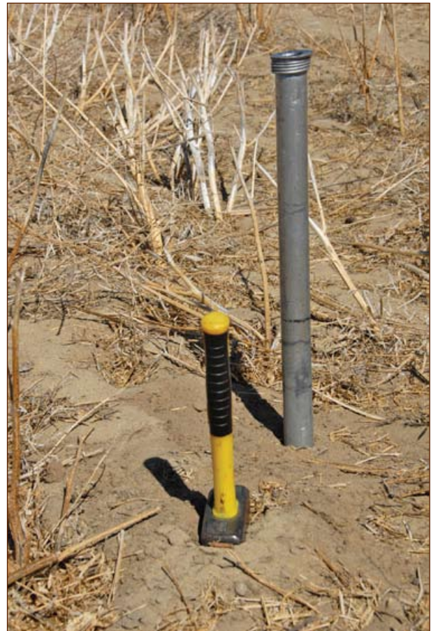
Figure 5 An exhaust tube marked in 10 cm increments is useful for do-it-yourself sampling.
