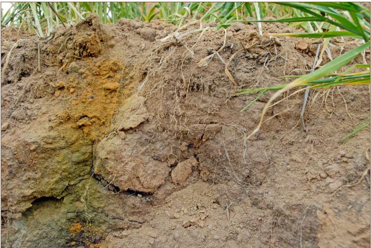
Figure 52 Soil profile stained with universal indicator at Hyden—the orange colour indicates an acidic layer at about 10–20 cm. Soil profiles that have an acidic layer will usually be corrected quicker following liming than a profile which is acidic to depth.
