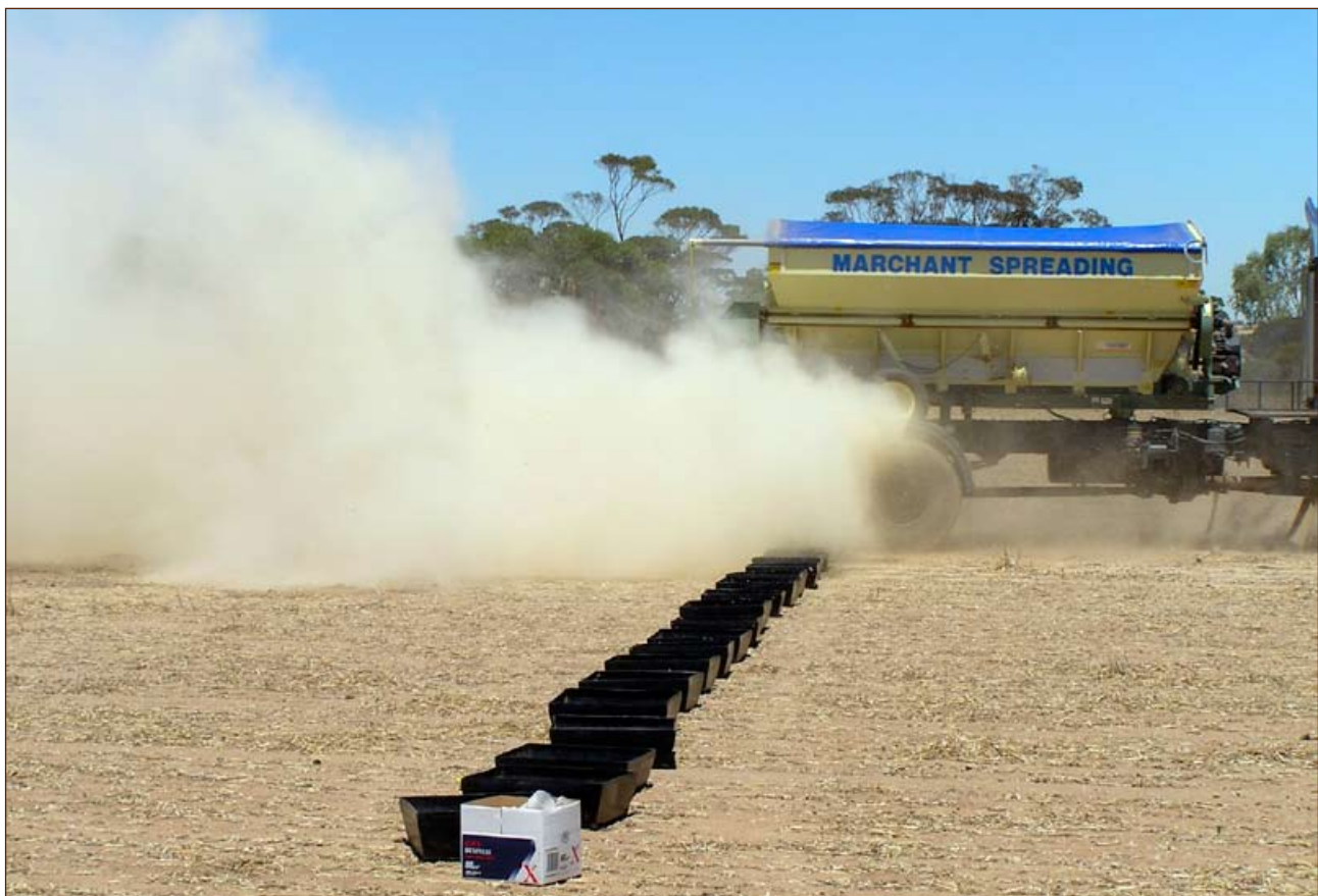
Figure 49 Testing agricultural lime spreading. Photo: D York
