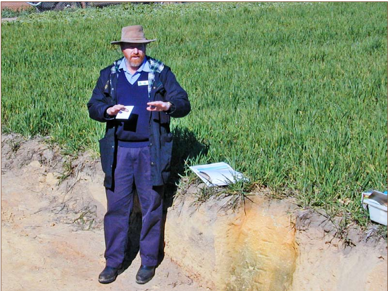
Figure 8 Soil profile stained with universal indicator at Tammin shows an acidic subsurface layer, stained orange, which would not be detected by only sampling topsoil
