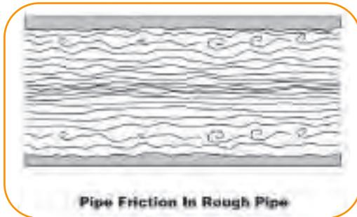
If the inside of a pipe is rough, the turbulence created restricts the velocity of water close to the pipe wall. Using a smooth bore pipe, this pipe friction results in lower flows and higher pressure drop along the length of the pipe.
