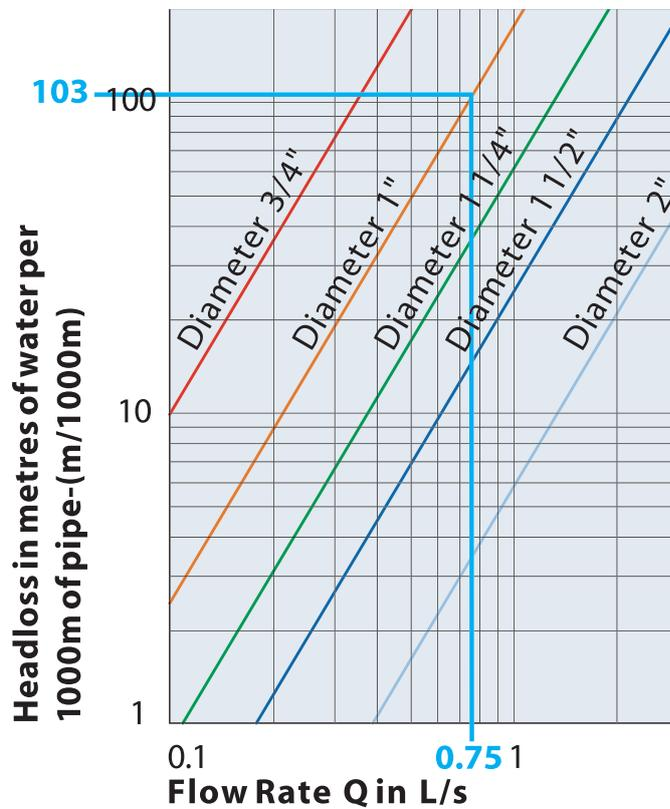
Use of the friction chart to determine head loss per 1,000m.
