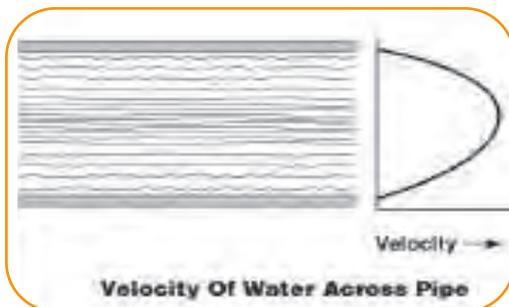
Because of friction created between water and the inner surface of a pipe, water across a pipe does not flow at even velocity. At the walls of the pipe the flow is close to zero, whereas at the centre the flow is the maximum. This can be likened to a river, where at the edge the flow is virtually zero due to friction created by the riverbank. The fastest flow will be in the middle of the river. This illustration shows a graph of velocity in relationship to pipe cross section.
