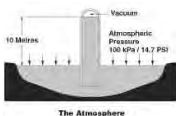
If a perfect vacuum is created in an inverted vertical tube, the atmospheric pressure on the surface of the water would push the water into the tube to a height of 10m.
