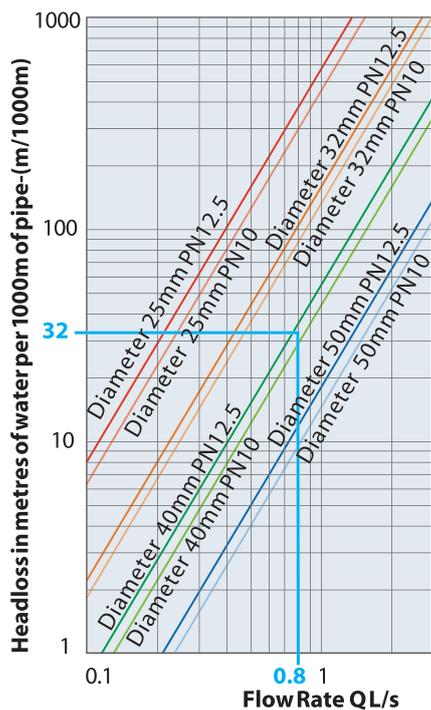
This chart shows that the nearest PN10 pipe to carry the desired flow rate of 0.8 L/s is a 40mm diameter pipe.
