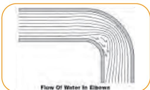
Due to centrifugal force and the shape of the elbow, the fluid flow is higher on the outside of an elbow. As the water is thrown to the outside surface, this effectively reduces the area in which the water flows. Sharp elbows create more centrifugal force increasing pipe friction, so it is good practice to use gradual radius bends where possible and keep the number of bends in any pipe system to a minimum to reduce the effects of friction.
