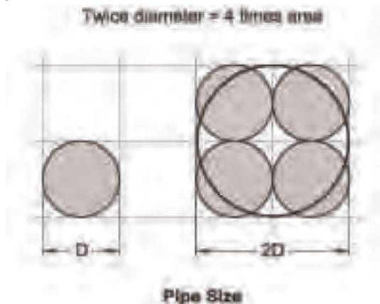
A small increase in pipe size increases the internal area of the pipe significantly. If the pipe diameter is doubled, the cross-sectional area increases by a factor of 4.
