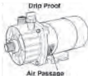
Drip Proof: usually quiet in operation, but dust, dirt, mice, snakes, frogs and other vermin can get into the motor through the cooling slots and cause it to fail.
