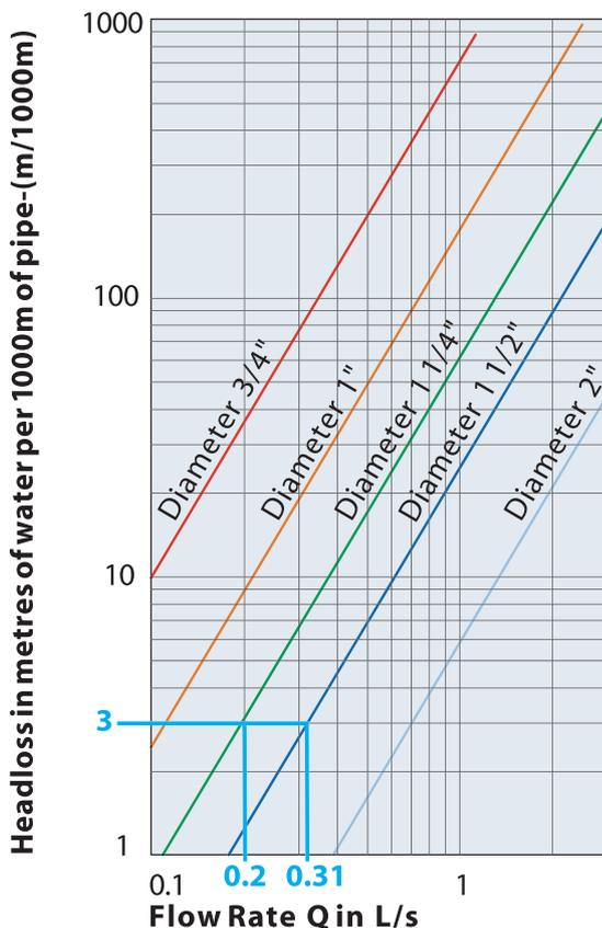
Under these conditions a 1 $\frac{1}{4}$ " pipe would give a flow rate very close to the required 0.2L/s. A 1 $\frac{1}{2}$ " pipe would give a flow rate of 0.31L/s.
