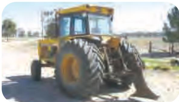
*Polyethylene pipe is fed down through the steel tube as the tyne is pulled through the soil by the tractor.*
