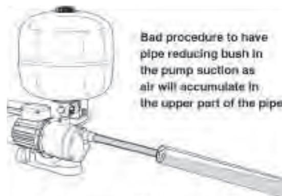
**Pipe connected to pump suction**
