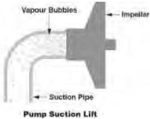
Water flowing in the suction pipe and entering the pump impeller can be extremely turbulent, releasing water vapour which can destroy the partial vacuum created by the pump.
