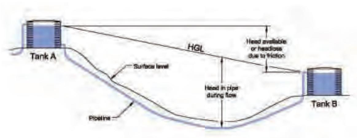
In the diagram (above) a tank on a hill has been used to provide the pressure to create flow. A pump may replace an elevated tank, particularly in flatter country. The pump raises the HGL in the same way as the elevated tank.
