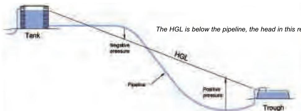
The HGL is below the pipeline, the head in this region is negative.
