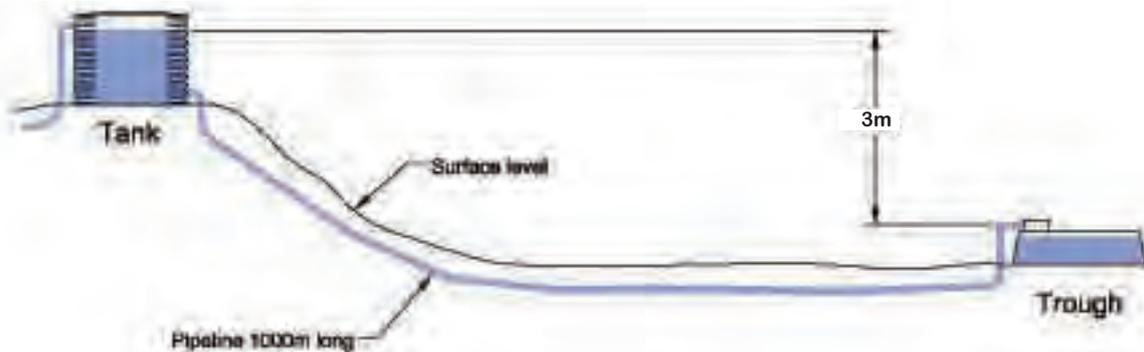
The trough is 1,000m from the tank; the available head is 3m. The HGL for this system is a straight line from the water surface in the tank to the outlet.
