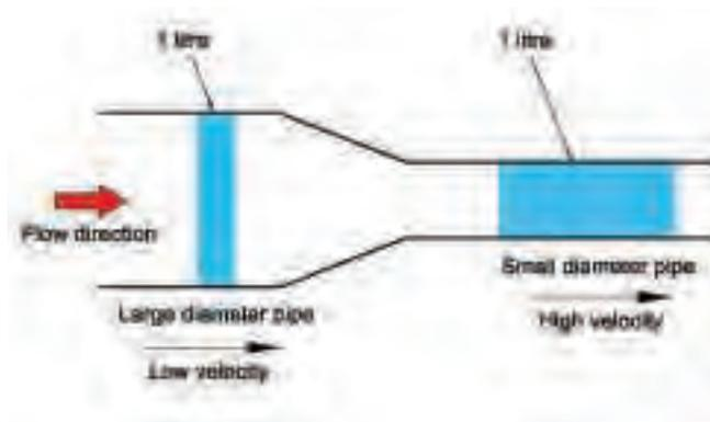
**For a given flow rate the smaller the cross-sectional area, the higher the velocity and therefore the higher the friction loss.**
