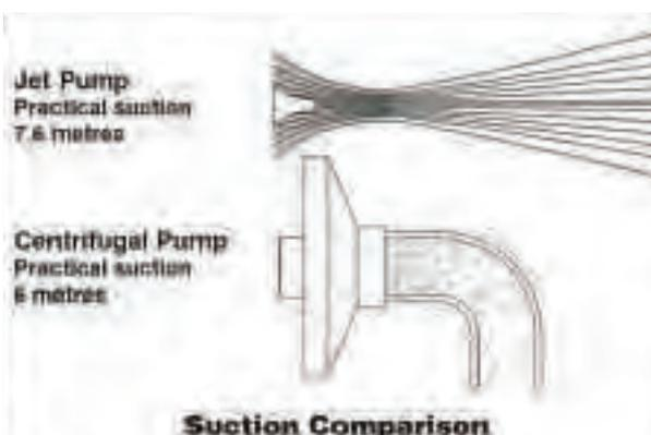
The jet pump is also versatile. By changing the venturi and jet assembly combination within the pump, the head and flow performance can be altered to suit the application.
