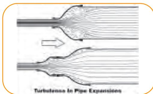
When a pipe is being increased or decreased in size, turbulence is experienced adding to pipe friction. Generally, keep expansion and reduction of pipe sizes to a minimum or at least in small steps if unavoidable.
