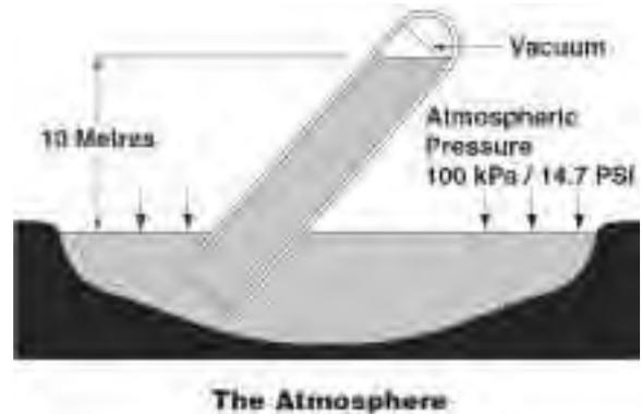
If this same tube is laid on an angle and again creating a perfect vacuum within, the atmospheric pressure would again push the water up the tube to a height of 10m.
