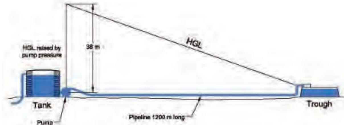
Available head is 38m, length is 1,200m, the flow rate is 0.8L/s.
