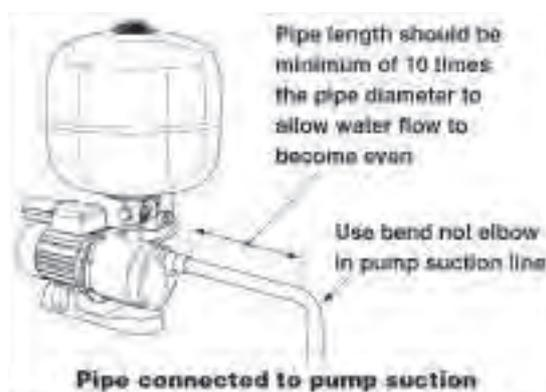
**Pipe connected to pump suction**
