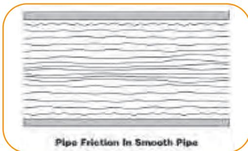
If a smooth bore pipe like PVC or polyethylene is used, there is less turbulence created and water velocity close to the pipe surface will be high; resulting in less friction and increased flow.
