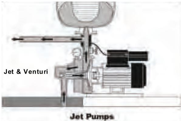
An injector containing a jet and a venturi added to the suction of a centrifugal pump increases the suction lift to between 7-8m and is known as a jet pump.
