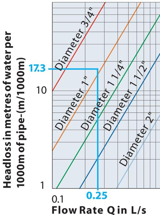
The friction chart above, shows that the nearest pipe size is 1 inch.
