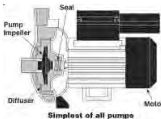
Centrifugal pumps are efficient, simple to maintain and are one of the most common pumps available.
