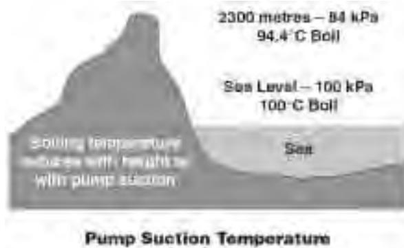
The temperature of water can affect the suction performance of a pump, and in the most extreme cases can even cause cavitation.
