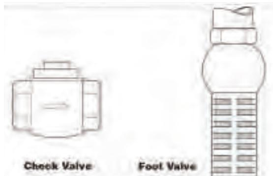
The check valve is also known as a one-way or non-return valve. The sole function of this valve is to stop any reverse flow.
