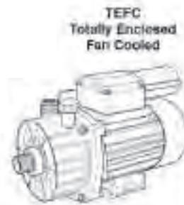
Totally Enclosed Fan Cooled (TEFC): the most common motor used to drive pumps. A more expensive motor to manufacture, but much more reliable.
