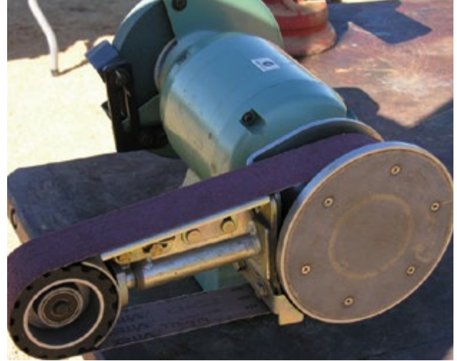
Photo 5.46 This Multi-tool 362 attaches to a 200mm bench grinder. PHOTO: Ian Evans
