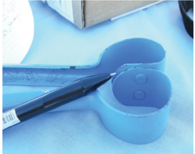
Photo 5.14 Bows mis-aligned. These shears are likely to be difficult to set properly. PHOTO: Ian Evans
