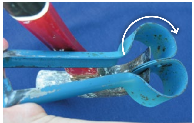
Photo 5.41 It will usually be necessary to twist the bow joint past the centreline a little to achieve centring when released. PHOTO: Ian Evans
