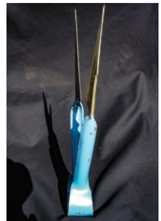
Photo 5.12 Too much tension between the blades. Often used to attempt to compensate for lack of set.
