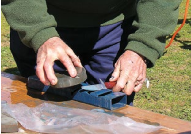
Photo 5.71 Using a jig will ensure a consistent sharpening angle. Note: The tip of this knife has been ground back for operator safety. PHOTO: Ian Evans
