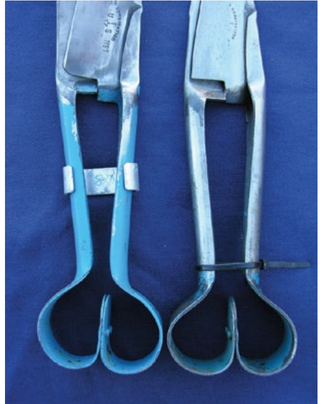
Photo 5.42 The shears on the left have a misaligned bow joint. The shears on the right are correctly aligned with knockers engaging equally. PHOTO: Ian Evans
