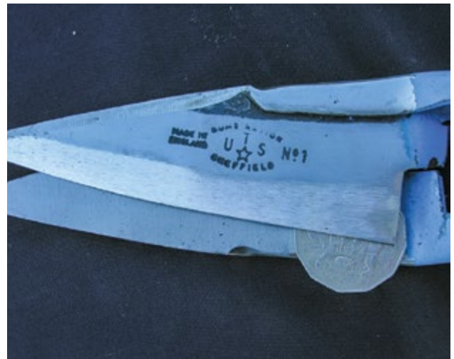
Photo 5.21 Well set, bent and open shears showing correct heel clearance. PHOTO: Ian Evans
