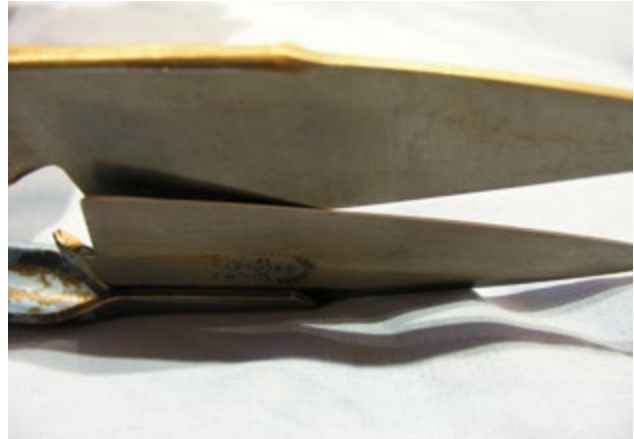
Photo 5.23 For an effective cutting action, the blades must lean towards each other so the cutting edges touch at only one point at a time. PHOTO: Ian Evans
