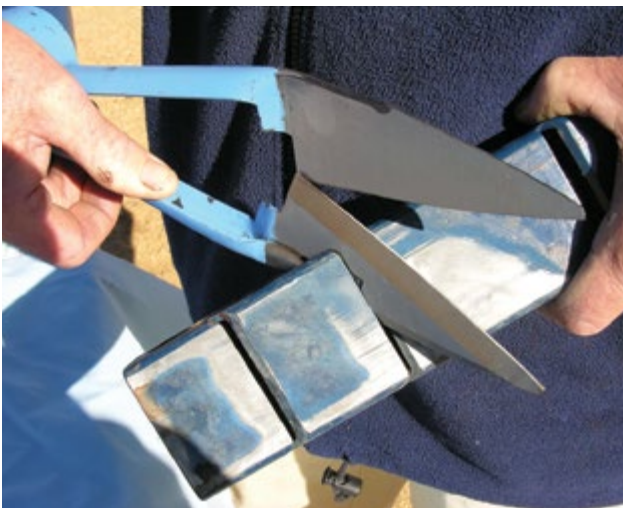
Photo 5.22 Setting blade clearance on right-handed shears using a sharpening jig. PHOTO: Ian Evans
