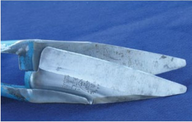
Photo 5.38 Knockers not correctly aligned and blade points uneven lengths due to bows and bow joint being out of shape. PHOTO: Ian Evans
