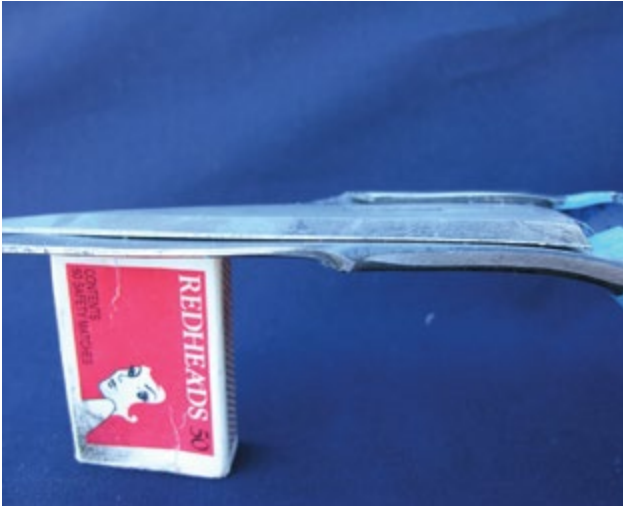
Photo 5.9 Insufficient gap at heel – no set. PHOTO: Ian Evans
