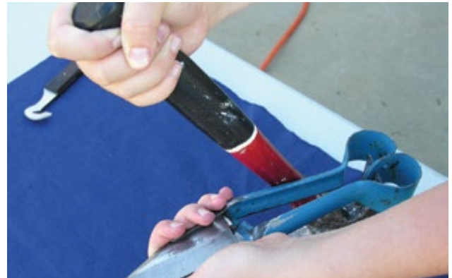
Photo 5.40 Use the claw of the hammer, to gently twist the bow joint back towards the centreline. PHOTO: Ian Evans
