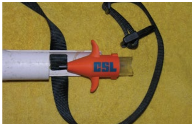
Photo 5.77 Another recoiling suspension system for a vaccine gun. Note: Vaccine pack is protected from direct sunlight and (partially) heat.
