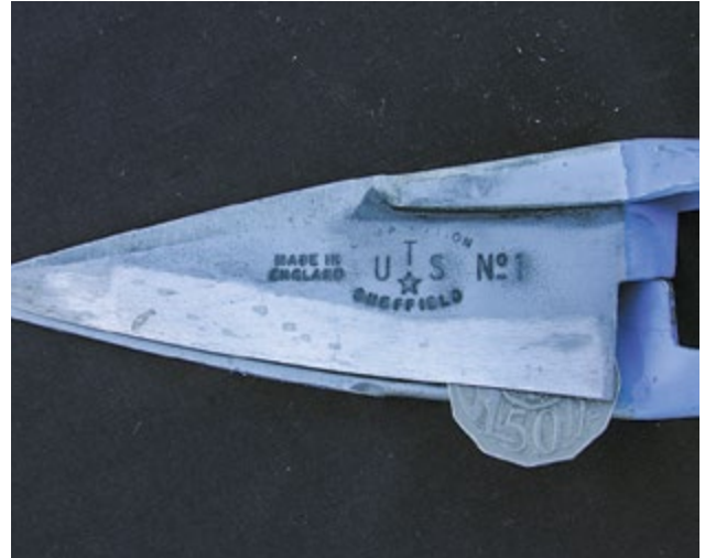
Photo 5.20 Well set, straight shears showing correct heel clearance. PHOTO: Ian Evans
