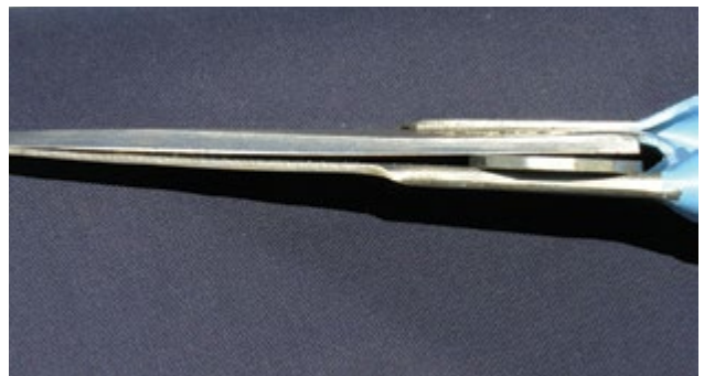
Photo 5.15 Ensure the clearance is greatest at the heels and could just allow a 50 cent piece (about 2mm thick) to slip in between the blades at the heels. PHOTOS: Ian Evans
