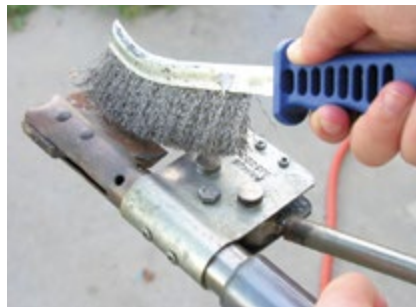
Photo 5.67 Keep the knife blade clean using a wire brush, always brushing away from the gas jet. Clean the gas jet with air and a solvent. It is advisable to carry two or three spare clean jets in a small, sealed container with other mulesing equipment. PHOTO: Ian Evans
