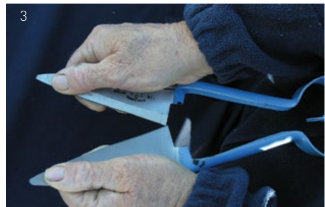
Photo 5.34 Holding a blade securely in each hand, gently push the blades with equal force in opposite directions. Do not hold one blade rigid and force the other away from it; remember equal force in opposite directions. Gloves provide protection, but reduce sensitivity. PHOTO: Ian Evans
