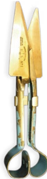
Photo 5.28 A clip can be used to keep shears closed. PHOTO: Ian Evans
