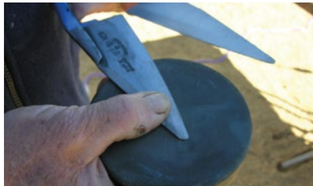
Photo 5.61 Remove the blade from the jig and while holding the stone flat against the inside face, draw the stone along the blade from the heel to the point only once. PHOTOS: Ian Evans
