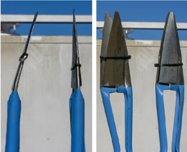
Photo 5.7 The use of bent (angled) or straight shears is a matter of personal preference. Mulesers who wish to maintain or set their own shears will need to develop high-level skills in setting and grinding. All mulesers need high-level sharpening skills. PHOTO: Ian Evans
