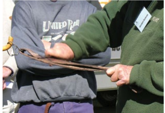
Photo 5.72 Knives can be polished with a leather strap. PHOTO: Ian Evans
