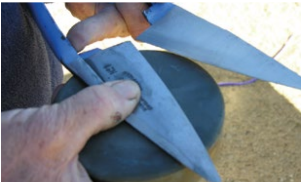
Photo 5.61 Remove the blade from the jig and while holding the stone flat against the inside face, draw the stone along the blade from the heel to the point only once. PHOTOS: Ian Evans
