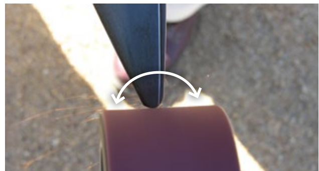
Photo 5.52 Grinding the points on 'closed-point' shears. For 'open-point' shears grind each point individually. PHOTOS: Ian Evans
