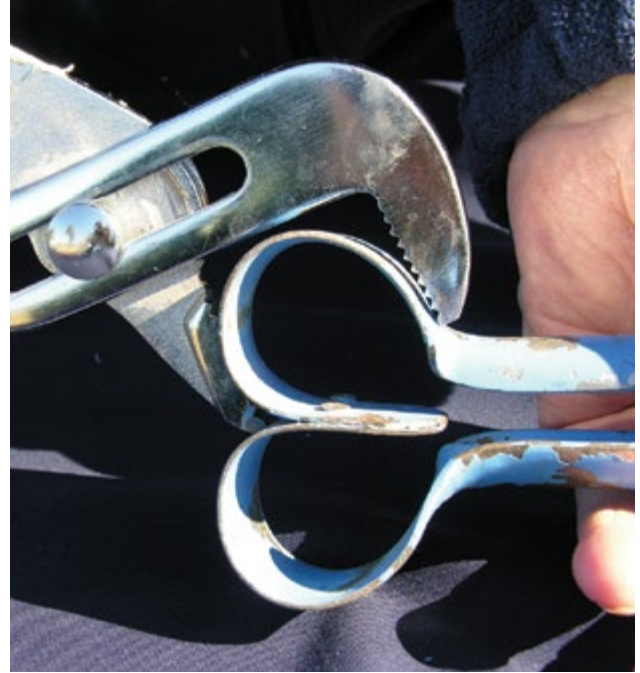
Photo 5.32 Remember to be gentle as the leverage of the multi-grips is enough to be easily crush the bow past the necessary point and out of shape. PHOTO: Ian Evans
