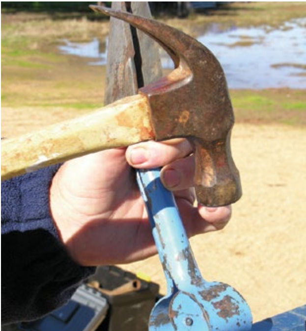
Photo 5.29 Use a hammer to gently hit the spot exactly where the handle meets the bow two or three times. PHOTO: Ian Evans
