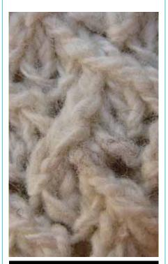
Single dark fibres in a white or pastel fabric need picking out at a cost of more than 10 cents per kilogram
