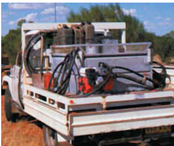
Figure 7. A well-equipped fire unit with a tank and reliable pump unit, hoses and adjustable nozzles, drip torches and UHF radio.
